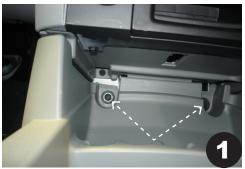
Remove (2) 10mm bolts underneath dash pocket.
