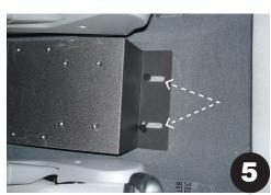
Using factory bolts, secure the backend of the Contour Console.
