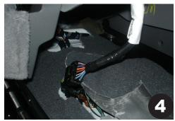
Slide driver's seat forward and lift up factory console. Unplug the console wiring harness. Remove console.
