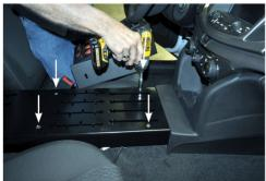
Remove (4) OEM screws using a 5/32 hex head driver.
