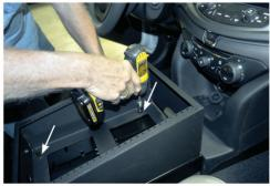
Using provided (4) socket button head cap screws, secure console into place. Short screws (2) in the back and long screws (2) in the front of console.
