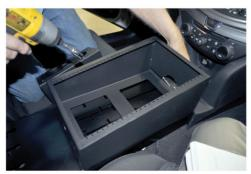
Place Jotto Desk Console on top of OEM floor plate, lining up holes of console with OEM holes.
