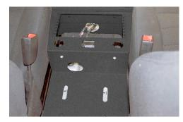
Accessory Adaptor Plate houses the OEM 12v outlets and USB connector. Utilize the provided USB extension cable. Plug the male end into the harness under the dash and the female end into the USB connector. Re-mount 12v outlets and USB connector into Accessory Adaptor Plate
