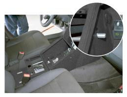
Secure Accessory Adaptor Plate to the front/face of Climate Control Console using provided hardware and to the rear mounting points using the OEM 8 mm screws.
