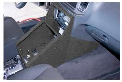
Position the console into the dash opening with the wings on the outside of the OEM dash sub-structure. Slots on floor of console should line up with OEM mounting studs. Work back toward dash to attain the exact position/fit.
