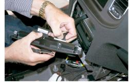
At this point – you need to remove the OEM Climate Control Cluster. At the bottom left and right edge, pull away from the dash and it will unsnap from the OEM dash structure. Disconnect cable from rear of CC cluster. Set aside for later use.
