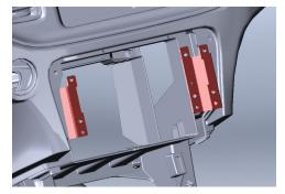
Attach the left and right radio brackets (brackets are stamped left/right) to dash in same location radio was removed from.
