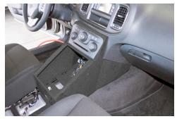
Install climate control into Jotto Desk Contour Console and connect cables back into module.
