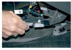
Disconnect wiring harness for 12V, USB, and Proximity Sensor from OEM console.
