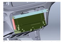
Re-install radio to radio brackets using (4) 10-32 screws. The cross brace attaches with the two upper screws.
