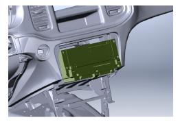
Remove OEM radio for relocation.
