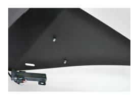
Relocate the Proximity Sensor to the driver's side wing of console using (2) 8-32 nuts. Place nylon washer, then sensor, then 8-32 nuts.
