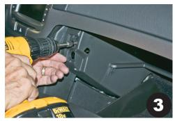
Remove plastic cover on left side as shown. Remove additional Phillips screw.
