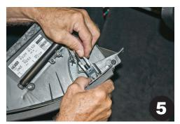
With glove box removed, detach light connection.
