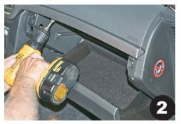
Open glove box and remove three (3) Phillips screws from top flange of glove box.
