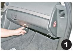
Begin by removing the two (2) lower Phillips screws from the bottom of the glove box.
