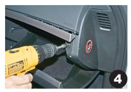
Remove plastic cover on right side as shown. Remove additional Phillips screw.
