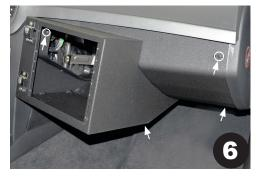
Install Console using four OEM Phillips screws as shown. Two (2) upper screws and two (2) lower screws.
