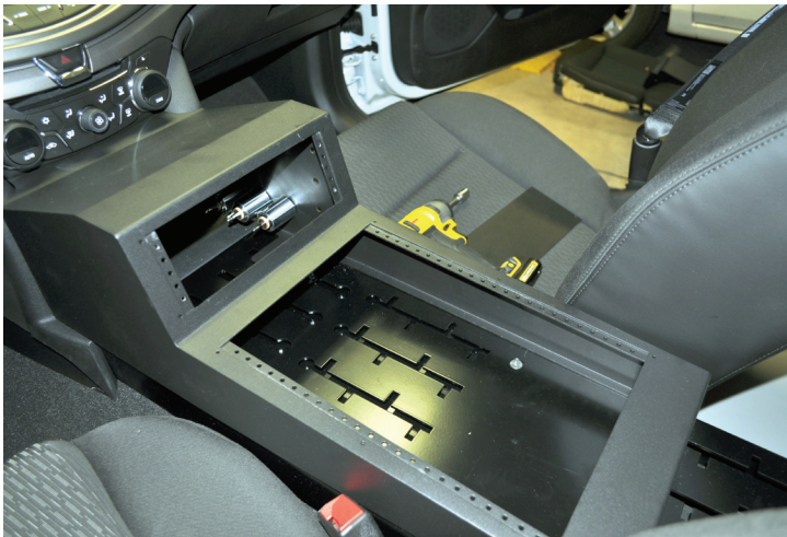
Place Contour Console on top of OEM console. Slide Contour Console snugly against the OEM dash.
