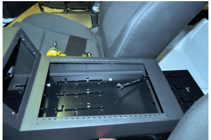
Secure Contour Console in place by sliding previously positioned carriage bolts into slots of console and tighten flange nuts using 7/16 socket.
