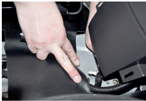
At dash of OEM cover plate – remove tab that secures a cable to OEM cover plate
