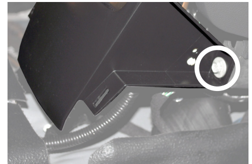
Remove Middle/Lower Dash Structure – by removing 2 (10 mm) bolts/screws.
