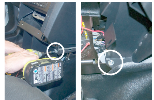
Attach Forward Mount Bucket using 8mm OEM bolts to upper location and 10mm OEM bolts to lower location.
