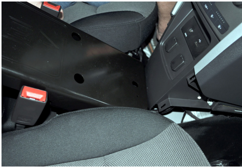
Remove all (6) 8mm bolts that secure OEM cover plate to vehicle (will be reused)
