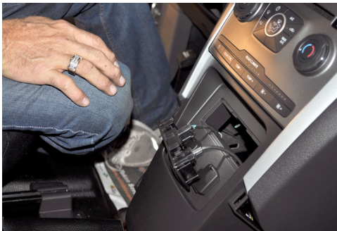
Disconnect (2) 12v outlets and USB/Line-in plate. Use small flat blade screw driver to remove OEM 12v outlets and USB/Line-in plate. Set aside for remounting USB in Jotto Desk Contour Console
