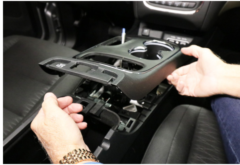
Pry up top/center OEM console. Disconnect all wires from top cover.
