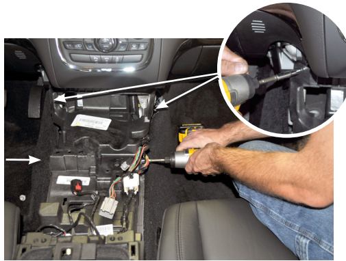
Remove (2) 10mm bolts and (2) 7mm bolts.
