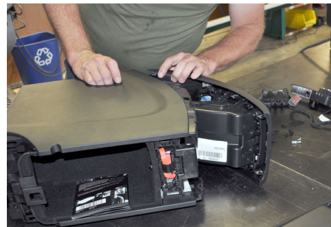
Now pry rear OEM cover from console.
