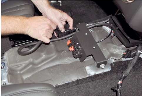
Attach Forward Mount Bracket into vehicle reusing (2) 10mm bolts. Once installed, route/connect Manual Park Release cable making sure that wire will not be pinched by Jotto Desk Contour Console. Note: See owner's manual section "What To Do In Emergencies" for more Park Release information.
