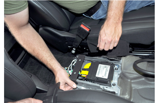
Attach Rear Mount Bracket with OEM (2) 10mm bolts.
