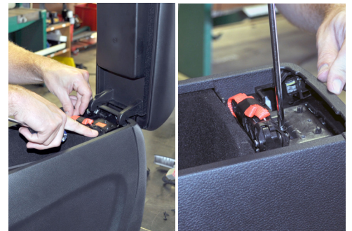
To remove Manual Park Release, you will need to remove (3) Phillips screws and set arm rest aside. Then remove (2) Phillips screws that are exposed.
