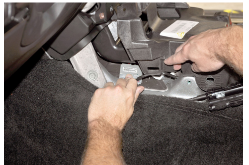
On the driver side of center console, unsnap Manual Park Release cable from OEM substructure.
