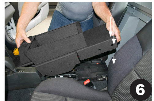
6 Install Caprice 9C1 MDC Console onto OEM center console, making sure that our brackets go inside of console/floorplate.
