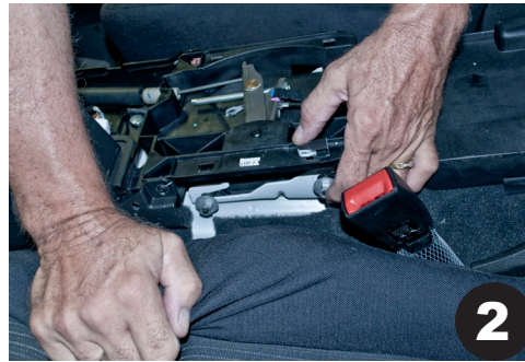
2 Remove 13mm nuts from the side of the transmission hump between seats and console. Two per side.
