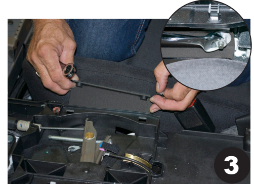
3 Install mounting brackets using provided 8mm hex nuts from previous step. Making sure to use the correct bracket on each side. Each should be marked P/S or D/S.
