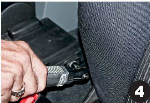
4 Remove 10mm bolts at the rear of the OEM floor plate. One per side.
