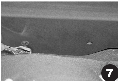
7 Attach front section using (2) 1/2" button head flange bolts through floor mounting plate into side mounting bracket. Repeat for other side.
