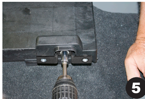
5 Install rear mounting brackets using the OEM 10mm bolts from previous step.
